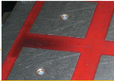
When different materials are used in the top face, due to shock/ heat and damage there is a chance of seepage of coolant/ liquid into the chuck, which results in burning of coil. Repair of coil is difficult, as no repair can begin without first destroying the chuck.
