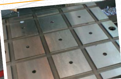
As the working face is made of single monolithic block of steel, inaccuracies due to unequal heating is reduced and there is no damage to the surface.
