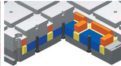
Coolant seepage is eliminated as the working face is of a single block of steel. In the unlikely event of coil burning, it can be easily repaired, after removing the bottom plate, without destruction of the chuck itself.
