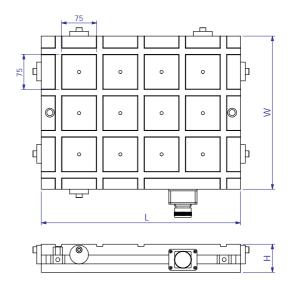
• The Magnet can be designed for 220/380/400/480 VAC, 50/60 Hz.
